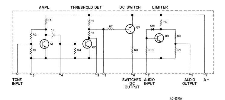
Figure 8 - Typical Threshold Detector Circuit
