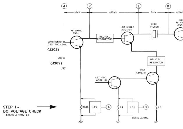
The DC voltage checks provide an easy method of checking the operation of the receiver stages with GE Test Set Model 4EX3A10 (or equivalent), and with no signal applied to the receiver.
