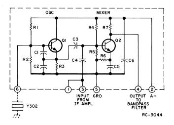
Figure 4 - Typical 2nd Mixer and Oscillator Circuit
