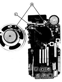
. When replacing the speaker in the mounting cup, align the two points (D). Route the speaker leads counterclockwise around the cup
