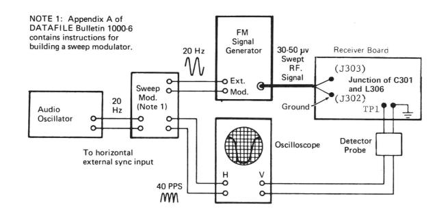
Figure 13 - Test Setup for 20-Hz Double-Trace Sweep Alignment
