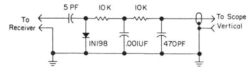
Figure 14 - Detector Probe for Sweep Alignment
