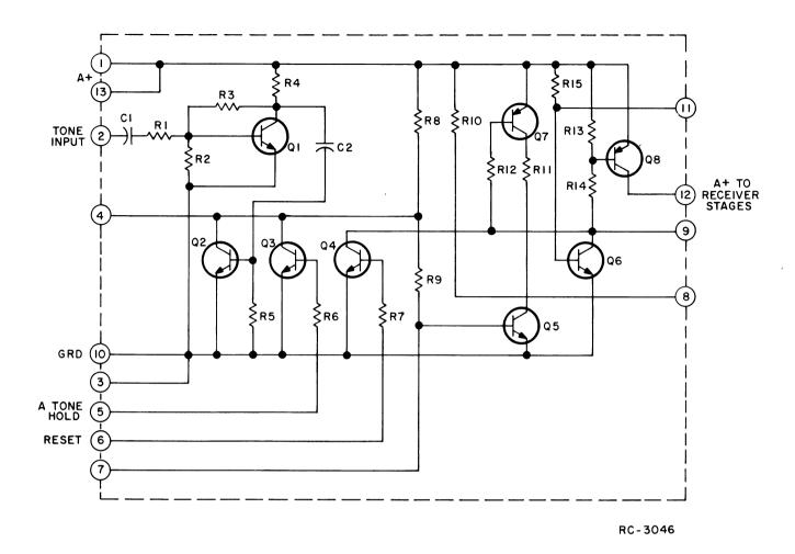
Figure 11 - Typical Battery Saver Circuit
