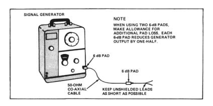
Figure 12 - Signal Generator Setup
