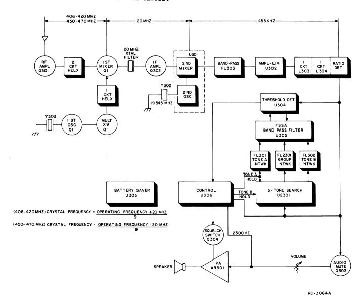
Figure 3 - Tone and Voice Receiver Block Diagram
