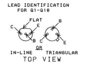
NOTE: LEAD ARRANGEMENT, AND NOT CASE SHAPE, IS DETERMINING FACTOR FOR LEAD IDENTIFICATION.
