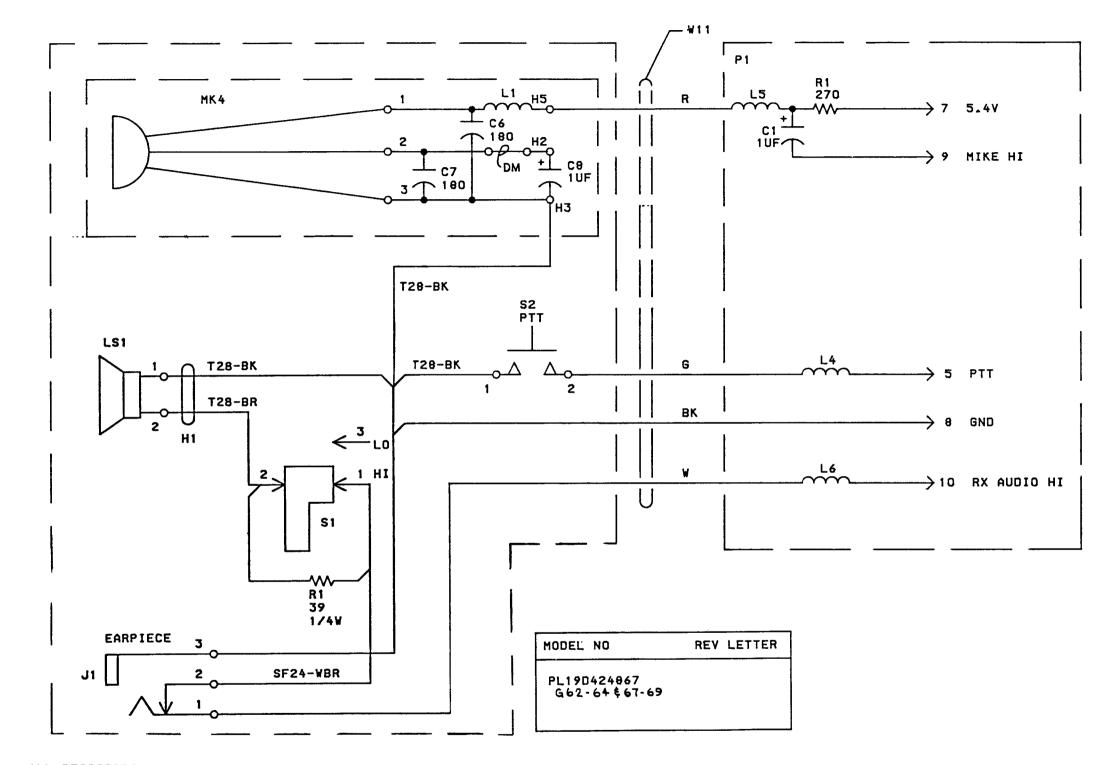
ALL RESISTORS ARE 1/4 WATT UNLESS OTHERWISE SPECIFIED AND RESISTOR VALUES IN OHMS UNLESS FOLLOWED BY K-1000 OHMS OR MEG-1,000,000 OHMS. CAPACITOR VALUES IN PICOFARADS (EQUAL TO MICROMICROFARADS) UNLESS FOLLOWED BY UF-MICROFARADS. INDUCTANCE VALUES IN MICROHENRYS UNLESS FOLLOWED BY MH-MILLIHENRYS OR H-HENRYS.
