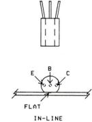
NOTE: CASE SHAPE IS DETERMINING FACTOR FOR LEAD IDENTIFICATION.
