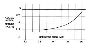
NOTE: DO NOT EXCEED THE CATH PA METER READING INDICATED IN THE CHART, FCC REGULATIONS PERMIT A POWER OUTPUT OF 50 WATTS; WITH A METER READING IN EXCESS OF THAT INDICATED IN THE CHART, POWER OUTPUT WILL EXCEED THAT PERMITTED.
