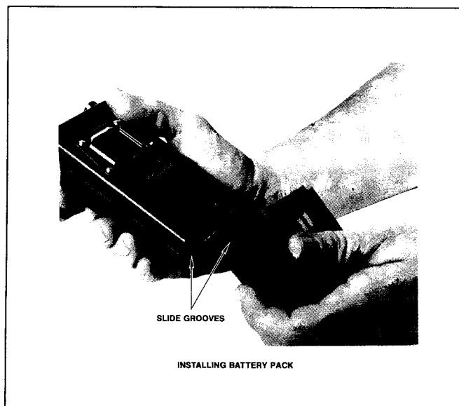
FIGURE 4 - INSTALLING THE BATTERY PACK
