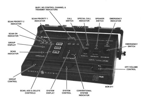
EMG (EMERGENCY) switch. Used to send an emergency message.
