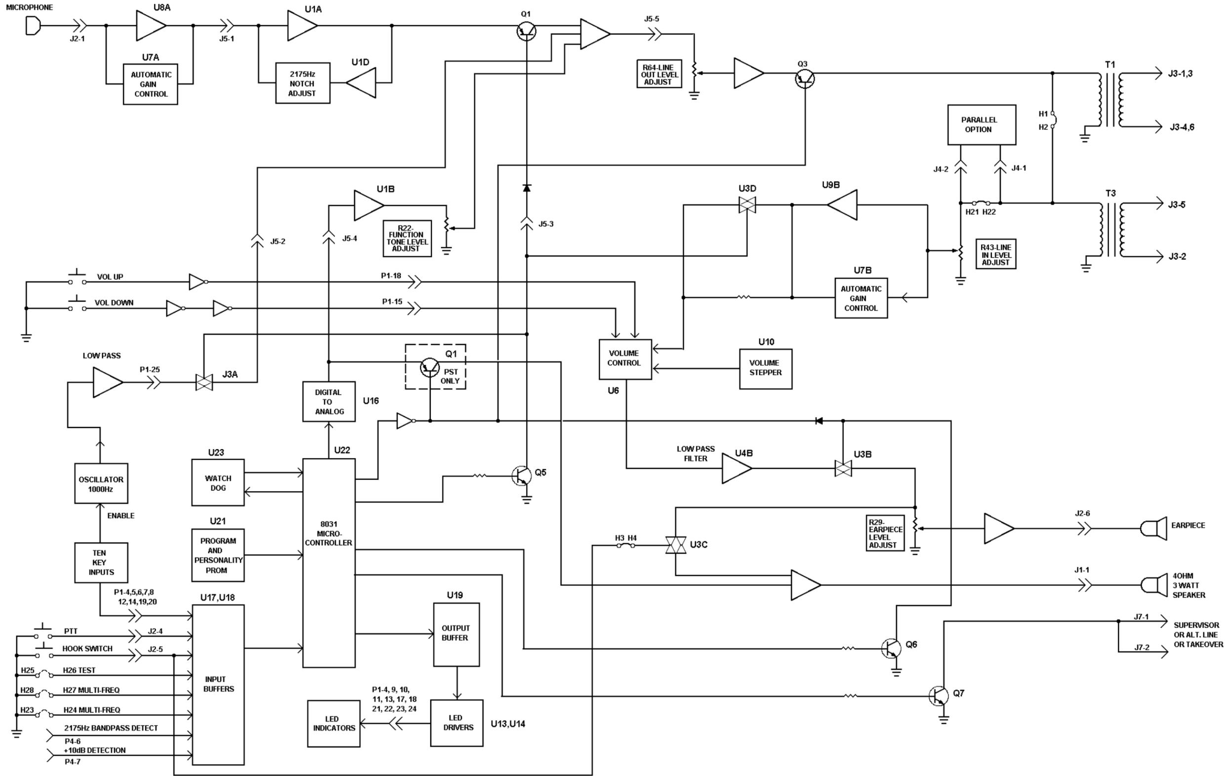
Figure 3 - EDACS RCN Block Diagram
