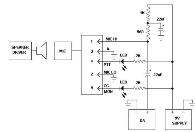
TEST CIRCUIT FOR MEASURING MICROPHONE RESPONSE
