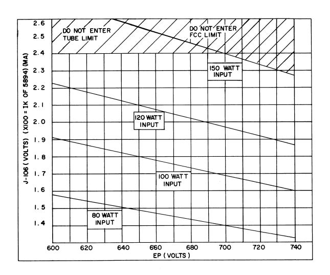
If the transmitter is to be used for continuous duty or long duty cycles, set the PA GRID drive from 0.1 to 0.2-volt higher than the peak power output reading. The required grid drive for the PA tube (5894) may vary from tube to tube.
