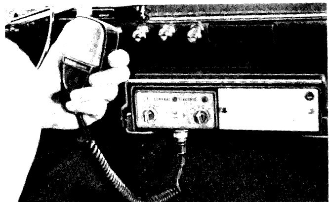
Fig. 3—Complete Two-Way Radio conveniently mounted near operator
