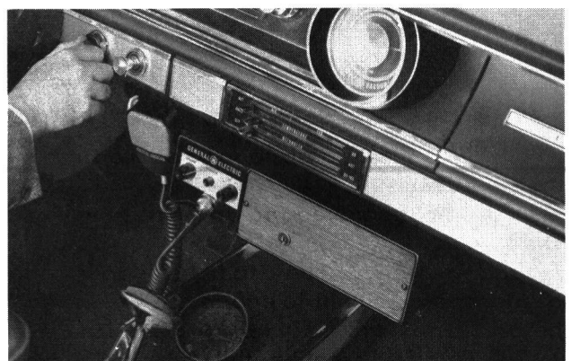
Fig. 4—Complete Two-Way Radio conveniently mounted near operator
