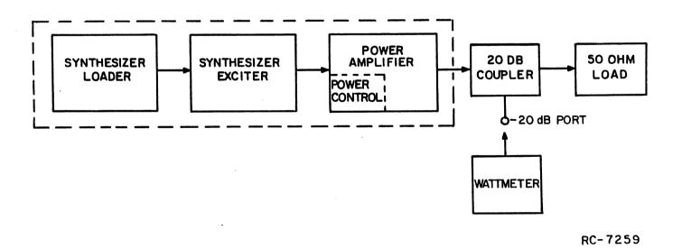
Figure 2B - Transmitter Test Setup
