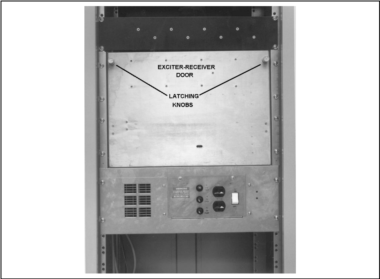
Figure 3 - Latching Knobs Securing Door
