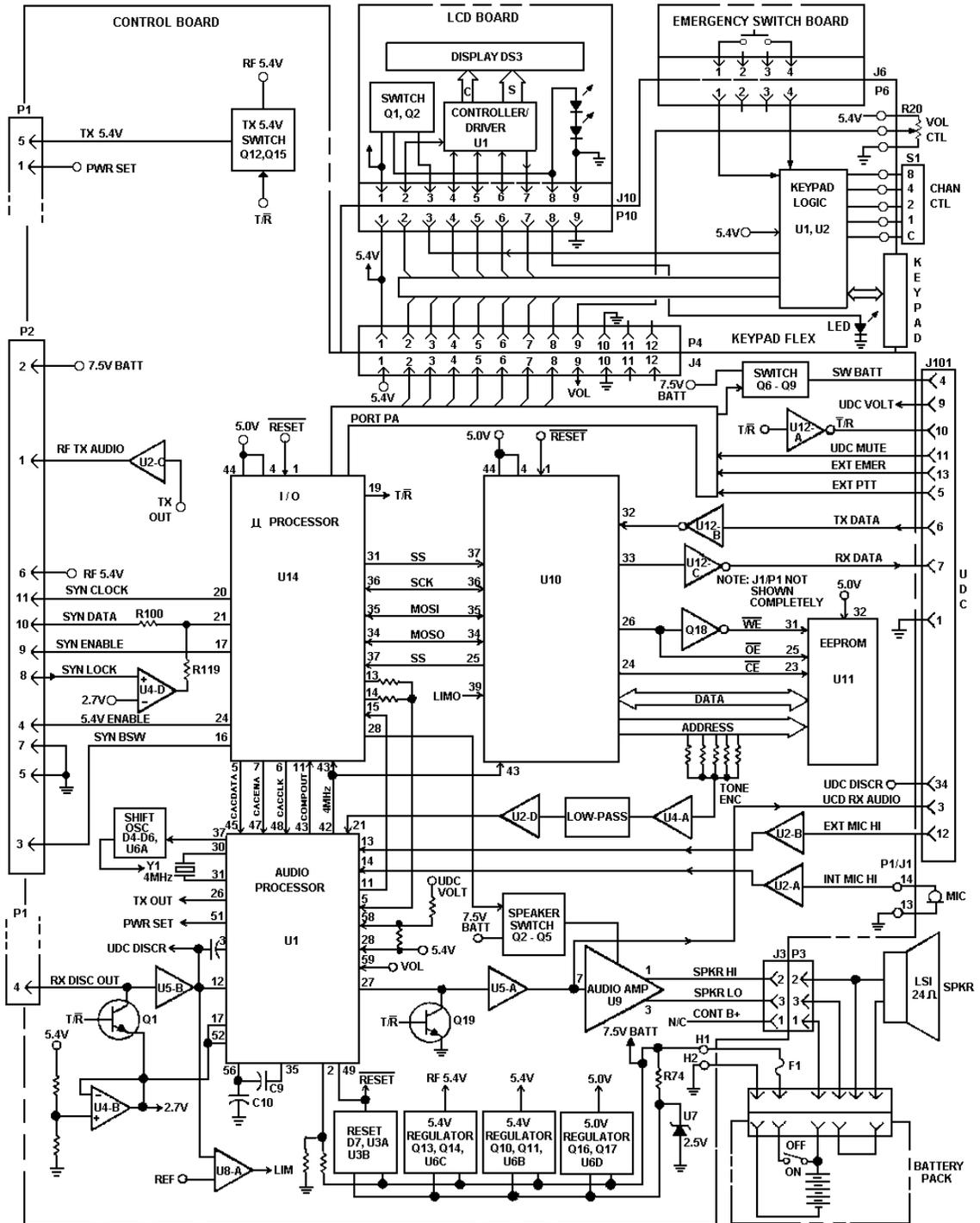
Figure 12 - Front Cover Assembly (Earlier) And Control Board Block Diagram
