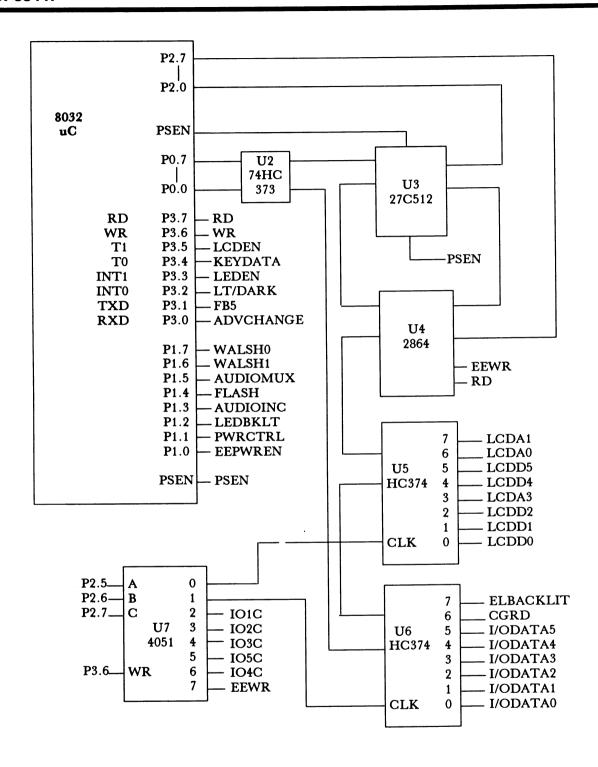
Figure 1 - Digital Block Diagram
