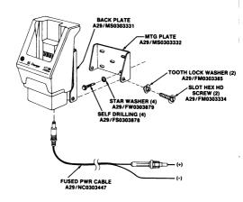
Figure 3 - Typical Mounting Configuration
