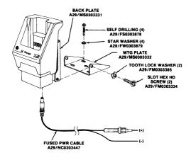
Figure 4 - Typical Mounting Configuration
