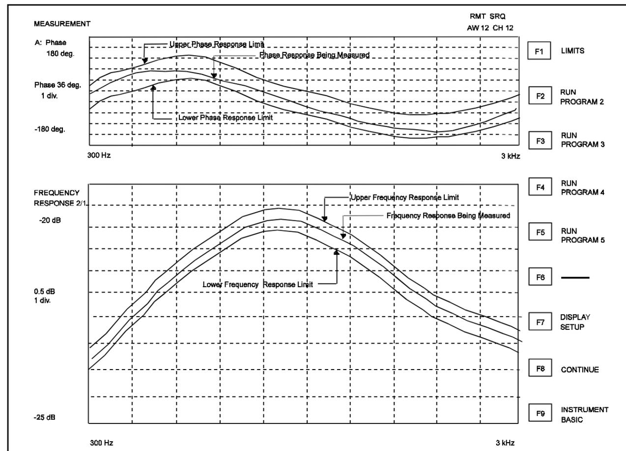
Figure 12 - Equalization Alignment Waveforms
