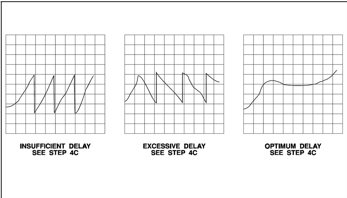
Figure 7 - Delay Waveforms
