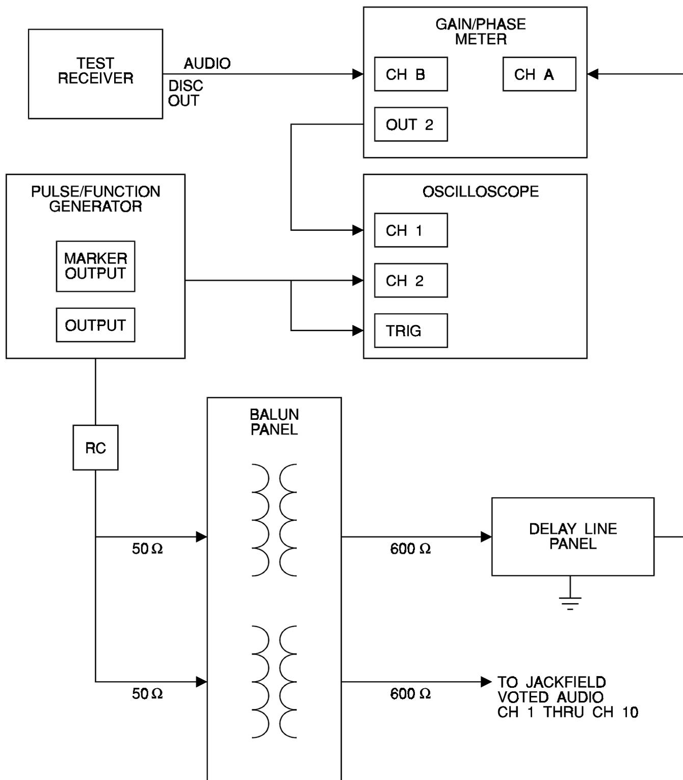
Figure 5 - Phase Equalization Alignment
