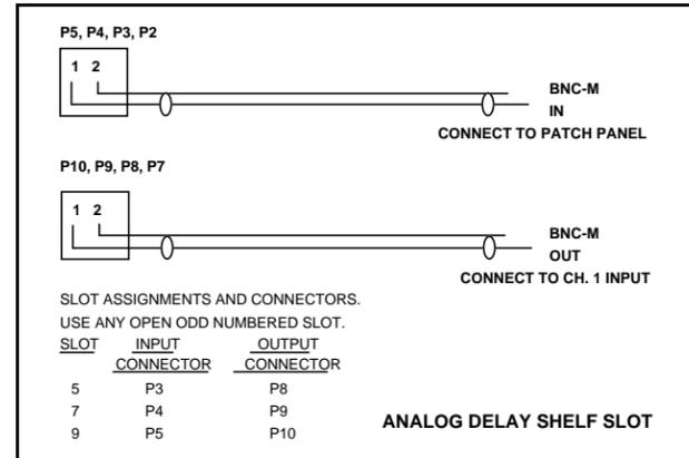
Figure 10 - Interconnect Cables, Analog Delay Backplane
