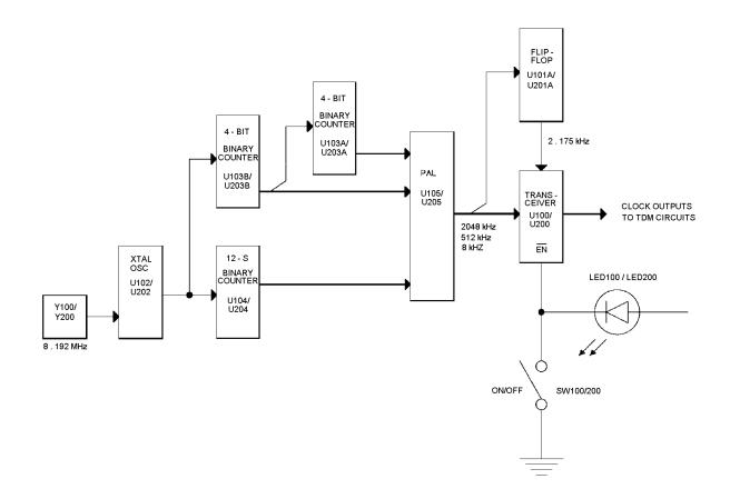
Figure 1 - Clock Board Block Diagram
