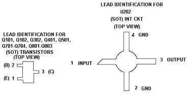
LEAD IDENTIFICATION FOR Q301 (SOT) TRANSISTORS (TOP VIEW) (B) 2 **5** (C) 3 5 (E) 1 5
