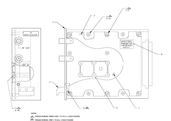
UHF TRANSMITTER SYNTHESIZER MODULE 19D902780G3, G6 - G10
