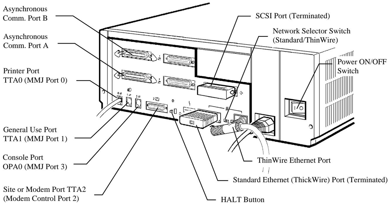
Figure 1-2. System Manager Model 85 CPU Cabinet (Rear View)
