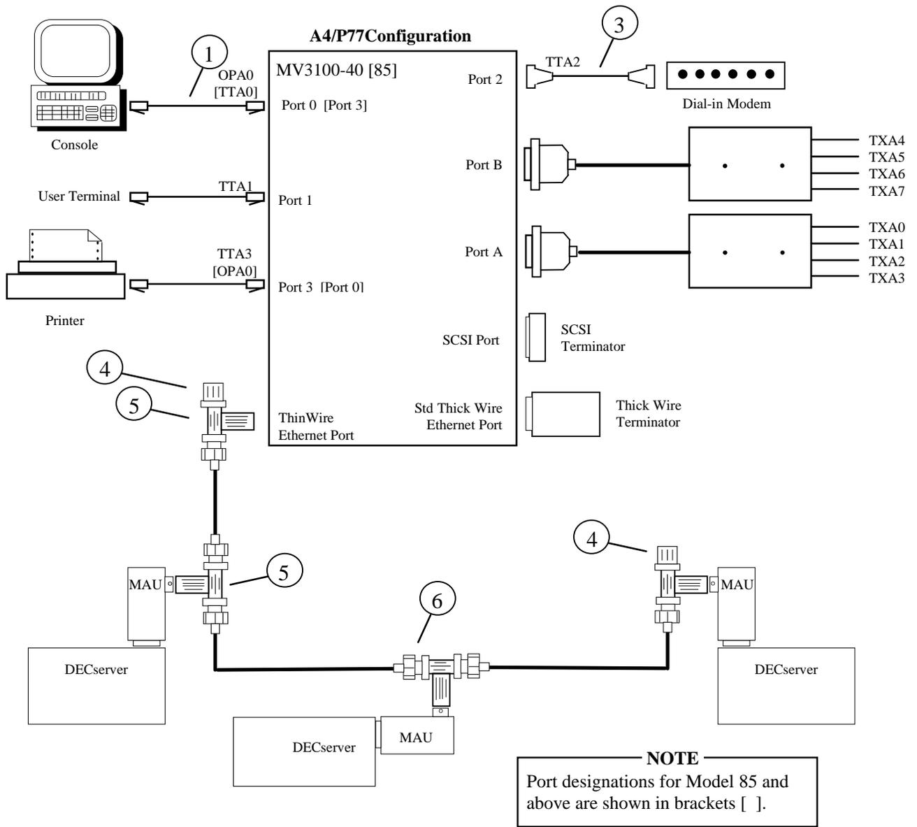
Figure 2-6. Typical A4/P77 System Configuration
