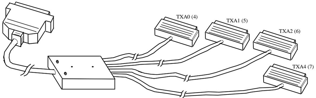
RS-232 Asynchronous Communication Interface Assembly (TXA Pods)
