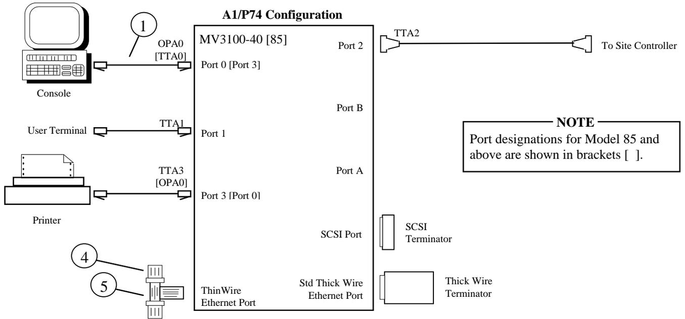
Figure 2-3. Typical A1/P74 System Configuration
