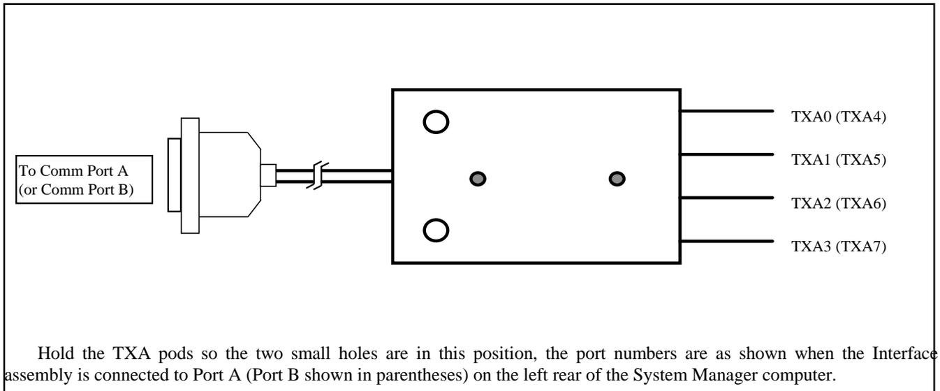
Figure 2-2. RS-232 Asynchronous Communication Interface Assembly (TXA Pods) Port Identification
