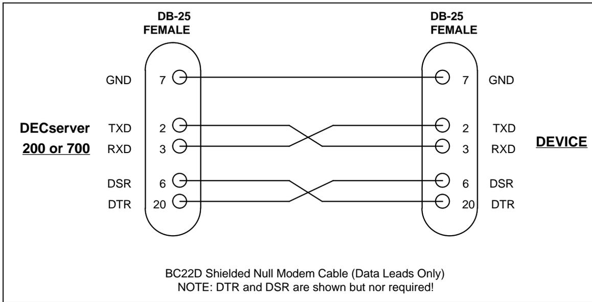
**Figure 2-8. Standard System Direct Connect Cable (RS-232)**
