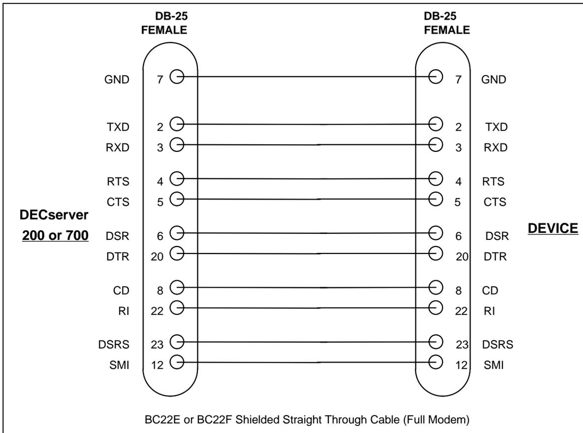
**Figure 2-9. Standard System Direct Connect Cable (RS-232)**
