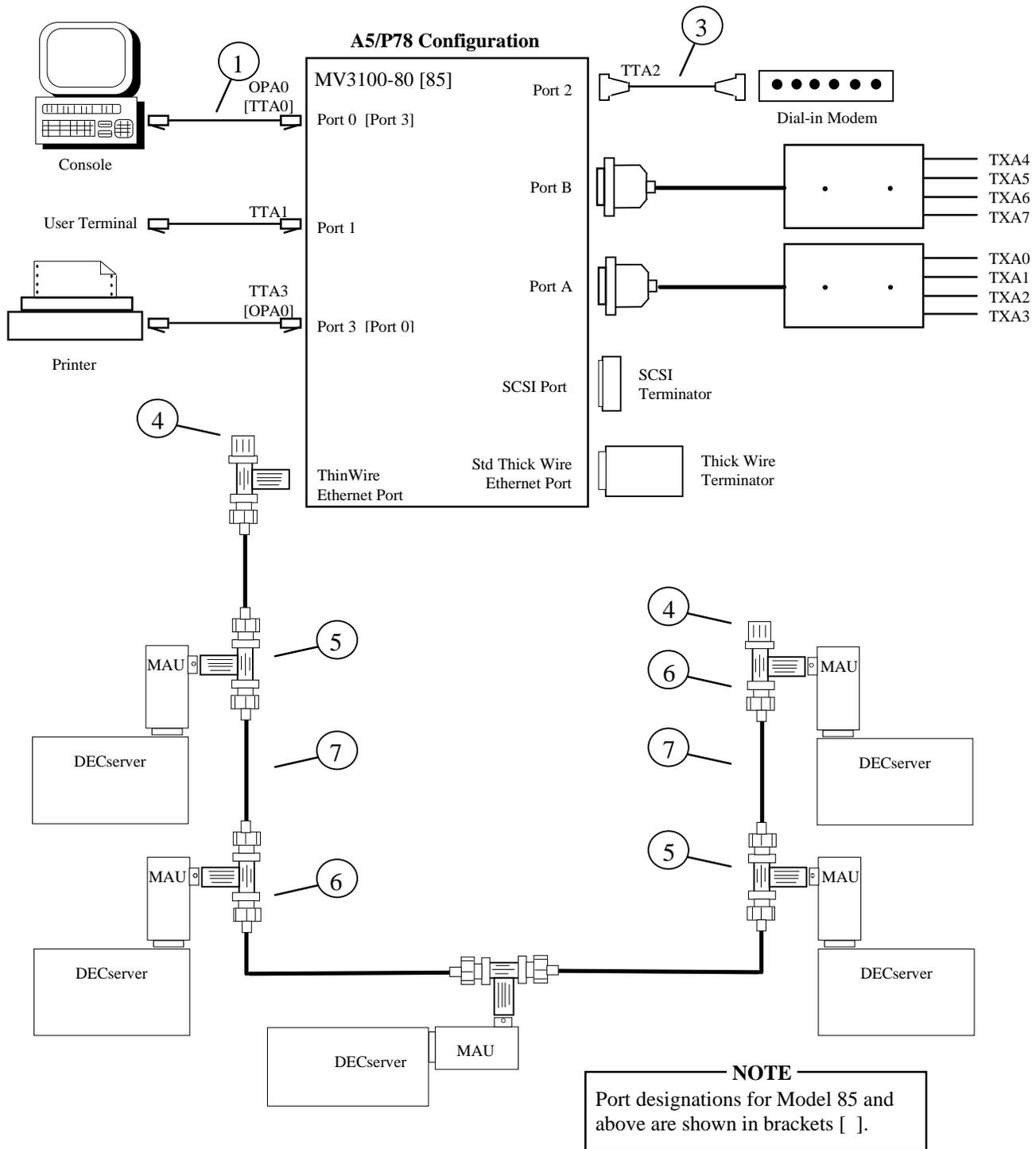
Figure 2-7. Typical A5/P78 System Configuration
