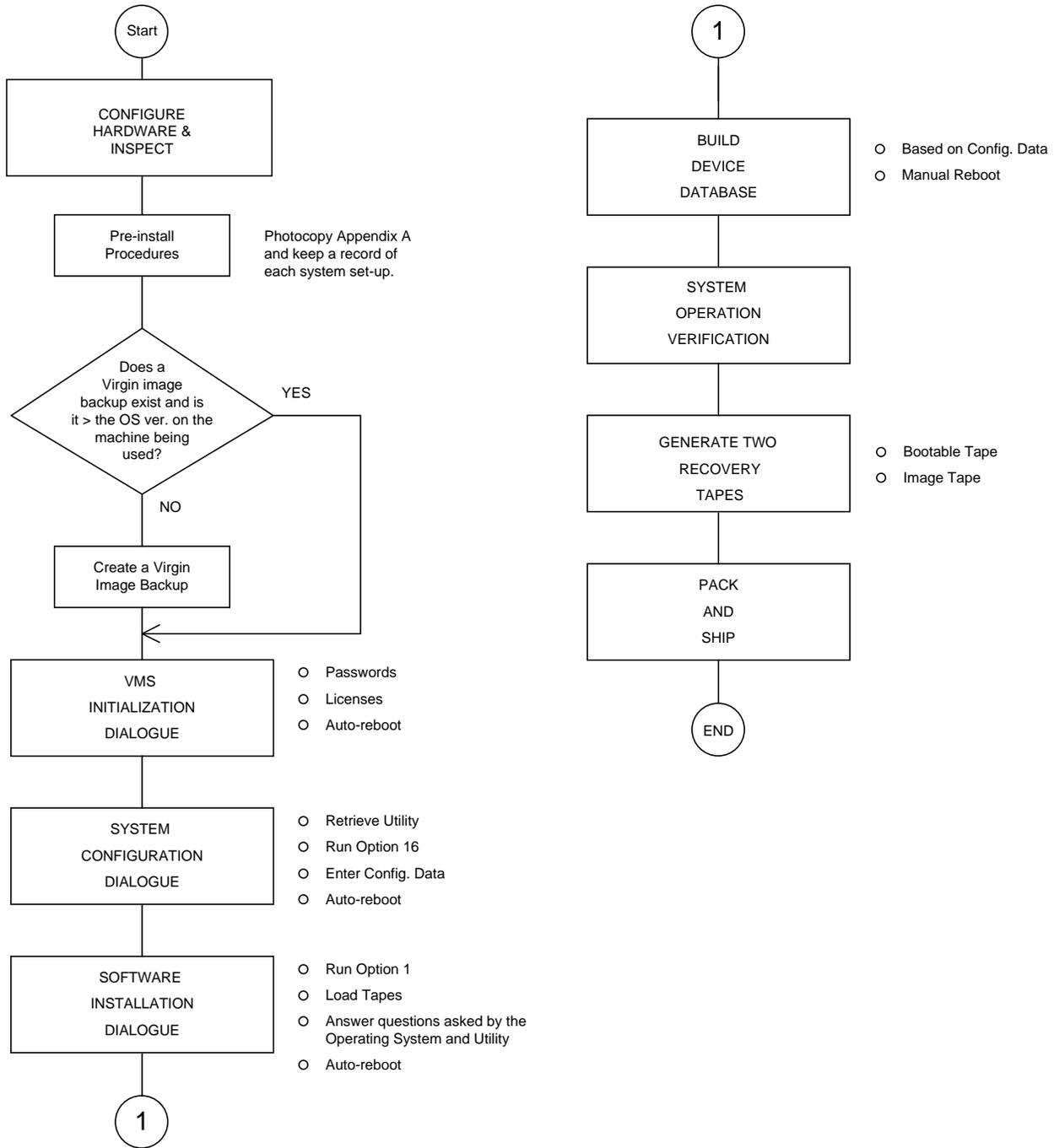
Figure 1-4. Initial Installation Process Flowchart
