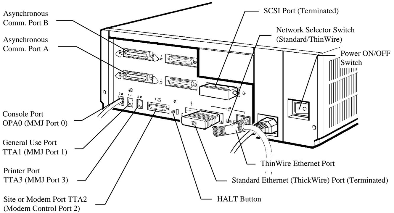
Figure 1-1. System Manager Model 40 and 80 CPU Cabinet (Rear View)
