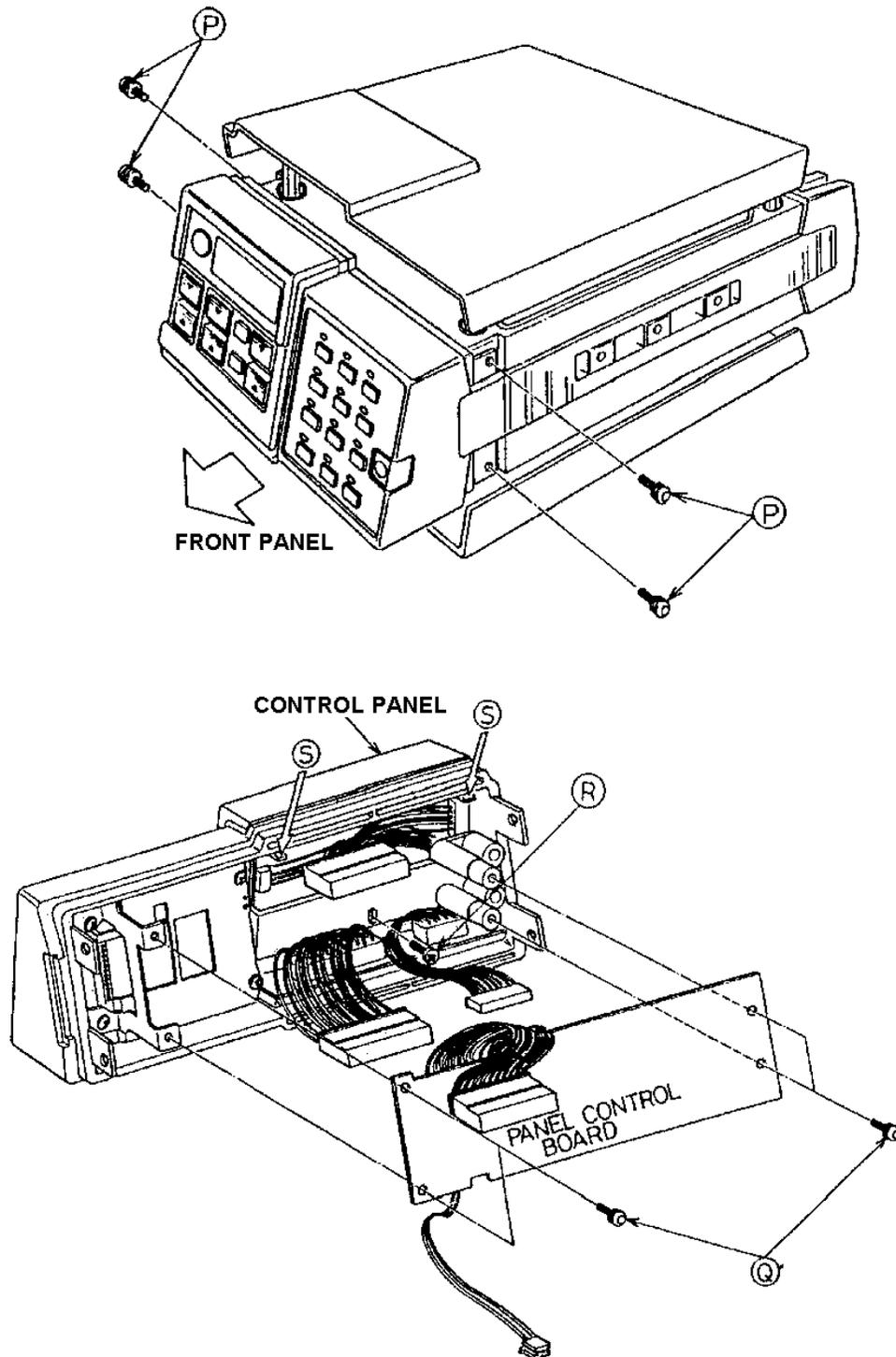
Figure 6 - Front Panel Disassembly
