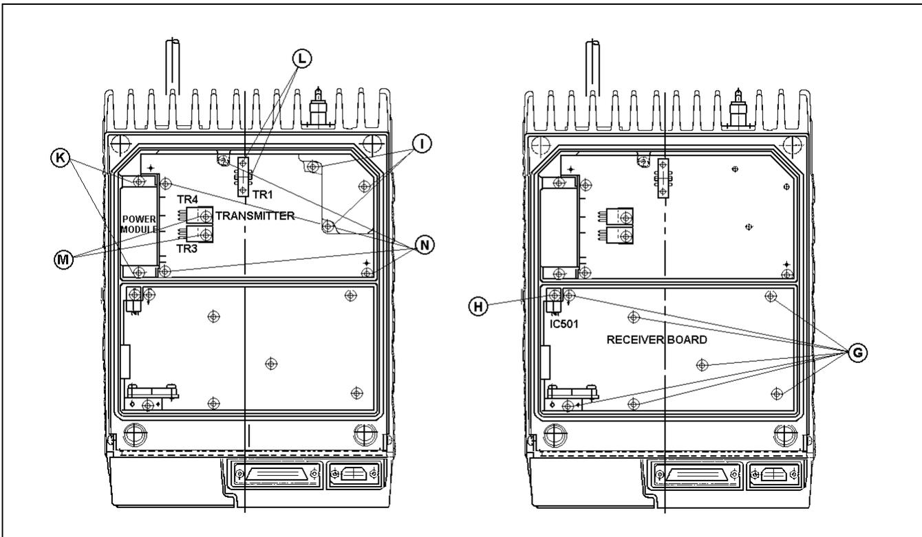
Figure 5 - Transmit and Receive Board Bottom View
