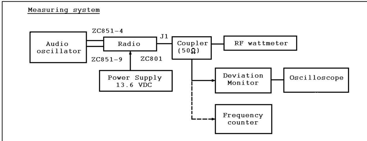
Figure 8 - Test Equipment
