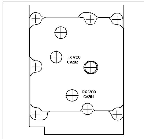
**Figure 10 - Adjustment Controls**
