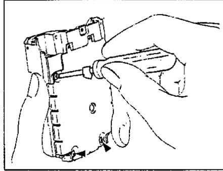
3. Remove the two screws (BIND, M2.6X6) on the side of the CASTING with the screwdriver and remove the PA MODULE RETAINER.
