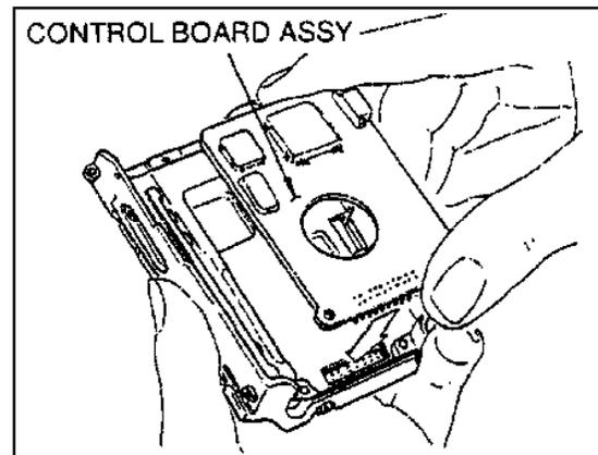
6. Secure the CONTROL BOARD ASSY. in the CASTING by fastening the three screws (PAN-HEAD with the SW, M2X4) with the screwdriver.
