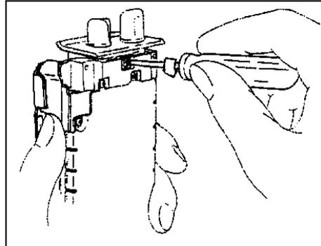
2. Loosen the two screws (PANHEAD, M2X2) on both sides of the LED FLEX ASSY. with the screwdriver and remove them.
