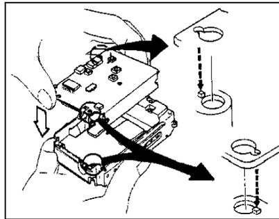
2. Install the RF SHIELD PLATE on the CASTING by fastening the three screws (PANHEAD with SW, M2X4) at the concave parts through the RF BOARD ASSY. with the screwdriver.
