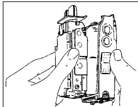
6. Disconnect the CONNECTOR A with a flat tipped tool.
