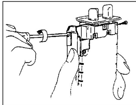
3. Insert a flat tipped tool into the frame of the CONNECTOR B as shown, and lift up the CONNECTOR B slightly to disengage the fitting.
