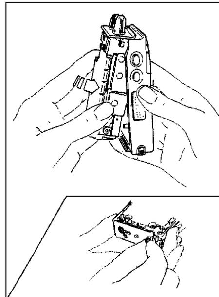
2. Secure the INTERNAL UNIT by fastening the two screws (PANHEAD, M2X6) at the upper part on both sides with the screwdriver.
