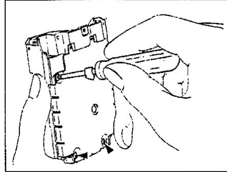
3. Remove the two screws (BIND, M2.6X6) on the side of the CASTING with the screwdriver and remove the PA MODULE RETAINER.
