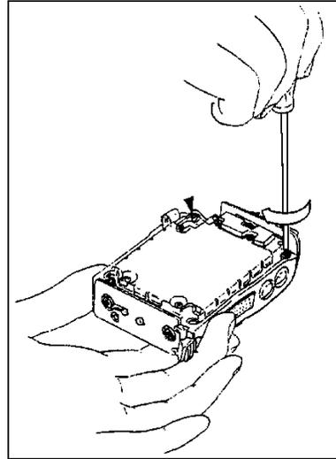
3. Fasten the two flat screws (M3) on the bottom of the FRONT CASE with the screwdriver.
