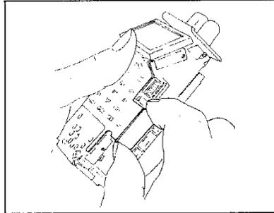
5. Insert a tool with thin end such as a minus screwdriver at the fitting between the LCD/KB FLEX ASSY. and the protruding part of the CHASSIS. Then disengage the fitting by twisting the tool, and remove the LCD/KB FLEX ASSY. gently.
