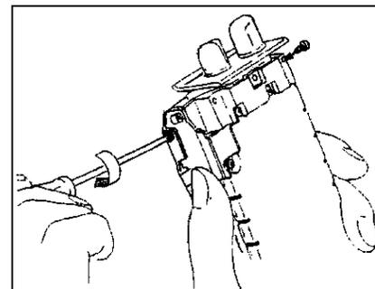
5. Fit the CONNECTOR B securely by pressing the FLEX P.C.B. on the CONNECTOR B with the thumb tip as shown.
