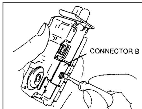
4. Hold the CONNECTOR B with your fingers and remove it taking care not to damage the connector pins.
