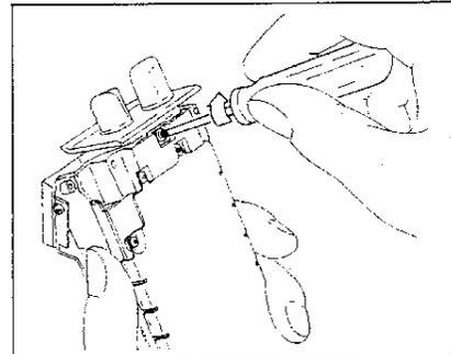
4. Secure the LCD/KB FLEX ASSY. by fastening the two screws (PANHEAD, M2X2) on both sides with the screwdriver.
