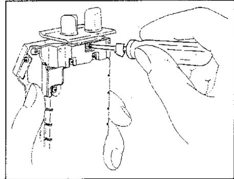
2. Loosen the two screws (PANHEAD, M2X2) on both sides of the LCD/KB FLEX ASSY. with the screwdriver and remove them.
