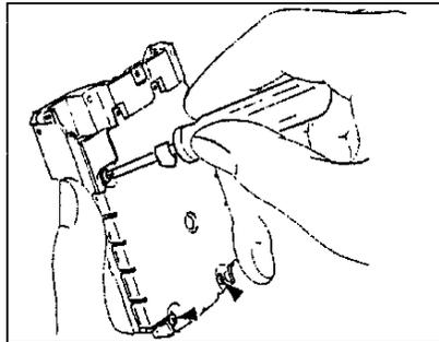
3. Secure the RF SHIELD PLATE by fastening the two screws (PANHEAD, M2X2) on the upper part with the screwdriver.
