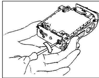
Note: After tightening screw, return the negative (-) battery contact (on the left side of diagram) just a little bit counterclockwise so the the contact is centered in the mounting groove.
