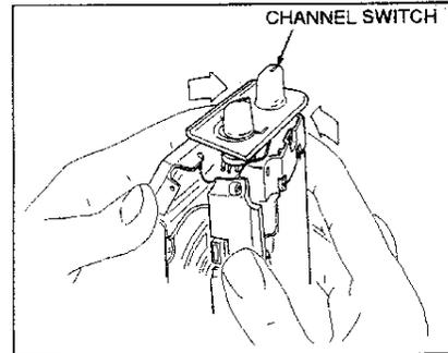
2. After engaging the upper part, fit the bosses of the LOGIC SHIELD PLATE with the holes on both sides of the CASTING.
