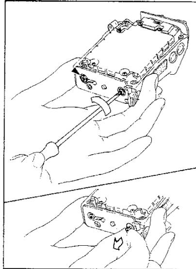
3. Loosen the two screws (PANHEAD, M2X6) on both sides at the upper part with the screwdriver and remove them.
