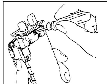
4. Secure the LED FLEX ASSY. by fastening the two screws (PANHEAD, M2X2) on both sides with the screwdriver.
