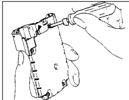
2. Remove the three screws (PANHEAD, M2X4 with SW) at the indented parts of the RF SHIELD PLATE, and remove the RF SHIELD PLATE.
