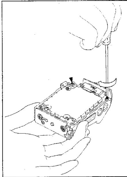
3. Fasten the two flat screws (M3) on the bottom of the FRONT CASE with the screwdriver.
