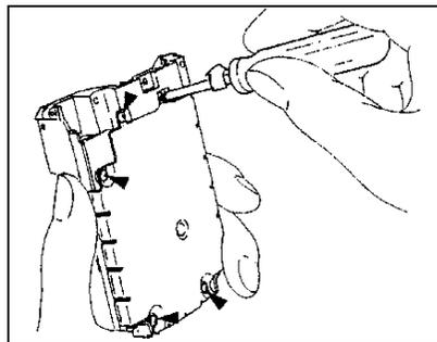
4. Insert the PA MODULE RETAINER into mounting holes and secure it by fastening the two screws (BIND, M2.6X6) on the side of the CASTING with the screwdriver.
