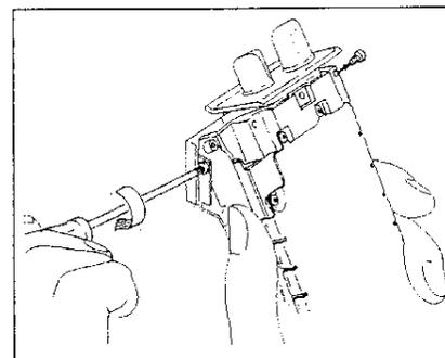
5. Fit the CONNECTOR B securely by pressing the FLEX P.C.B. on the CONNECTOR B with the thumb tip as shown.
