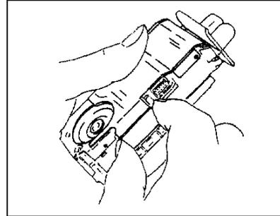
5. Insert a tool with thin end such as a minus screwdriver at the fitting between the LED FLEX ASSY. and the protruding part of the CHASSIS. Then disengage the fitting by twisting the tool, and remove the LED FLEX ASSY. gently.
