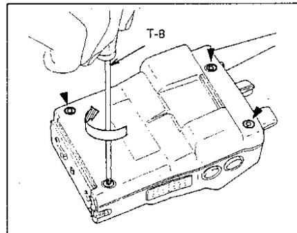
Note: Fastening torque should not be over 3.5Kg-cm.
