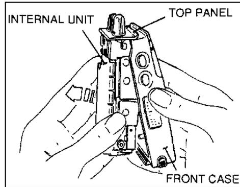
5. Remove the INTERNAL UNIT from the FRONT CASE being careful not to damage the FLEX P.C.B.
