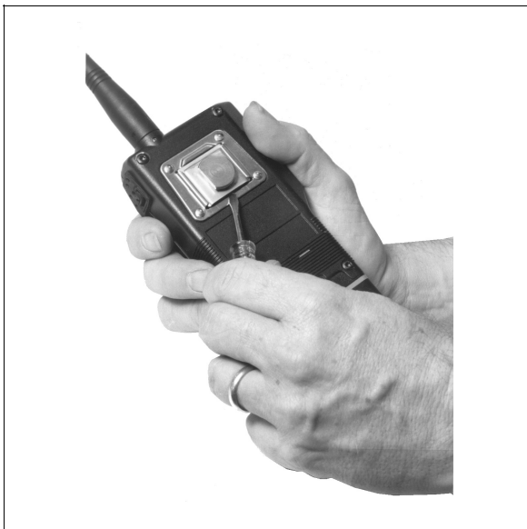
Figure 9 - Swivel Mount Removal And Replacement
