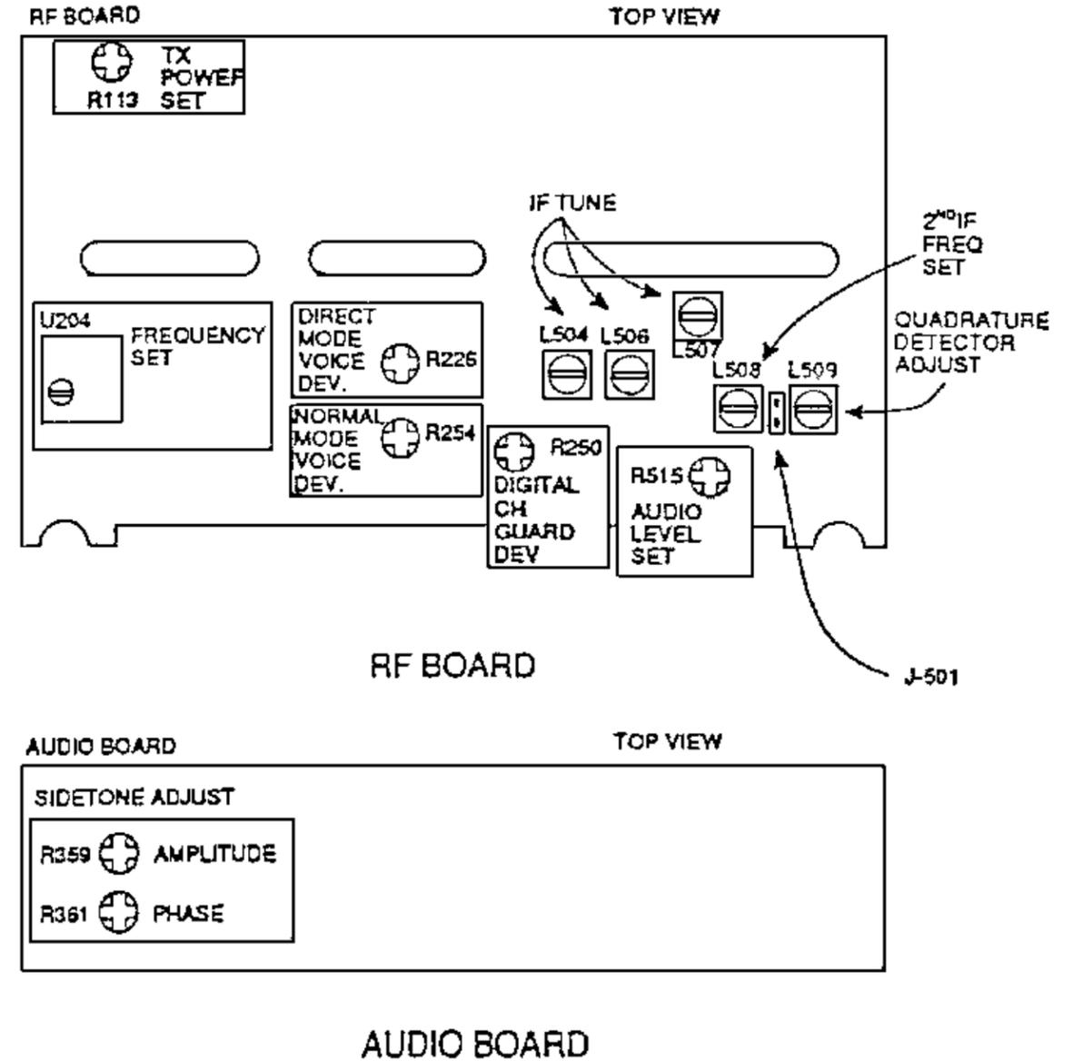
Figure 1 - Location Of Adjustment Controls
