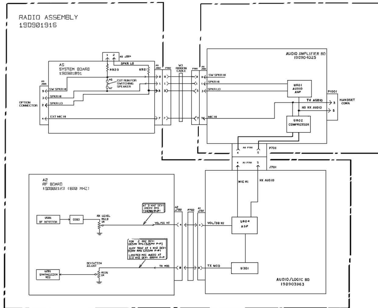
Figure 4 - Audio Signal Flow Diagram
