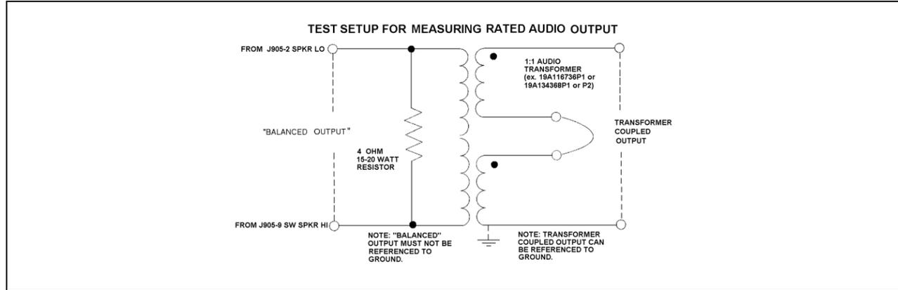
Figure 2 - Audio Output Test Set-Up Diagram
