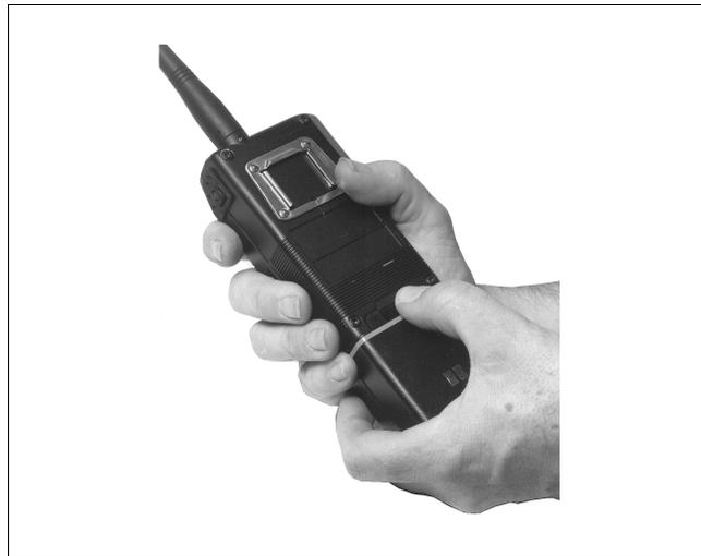
Figure 1 - Removing The Battery Pack
