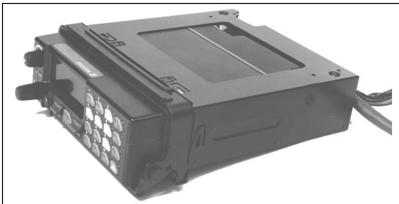
Figure 30 - Handle Assembly In LOCKED Position
