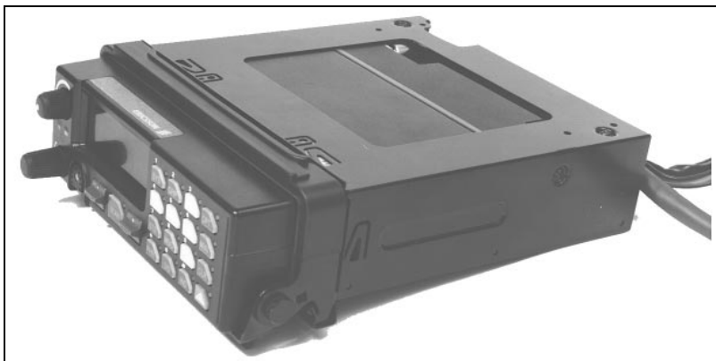
Figure 30 - Handle Assembly In LOCKED Position
