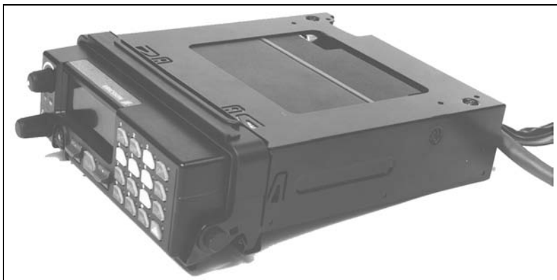
Figure 30 - Handle Assembly In LOCKED Position
