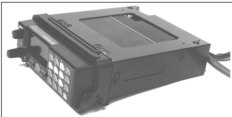
Figure 30 - Handle Assembly In LOCKED Position
