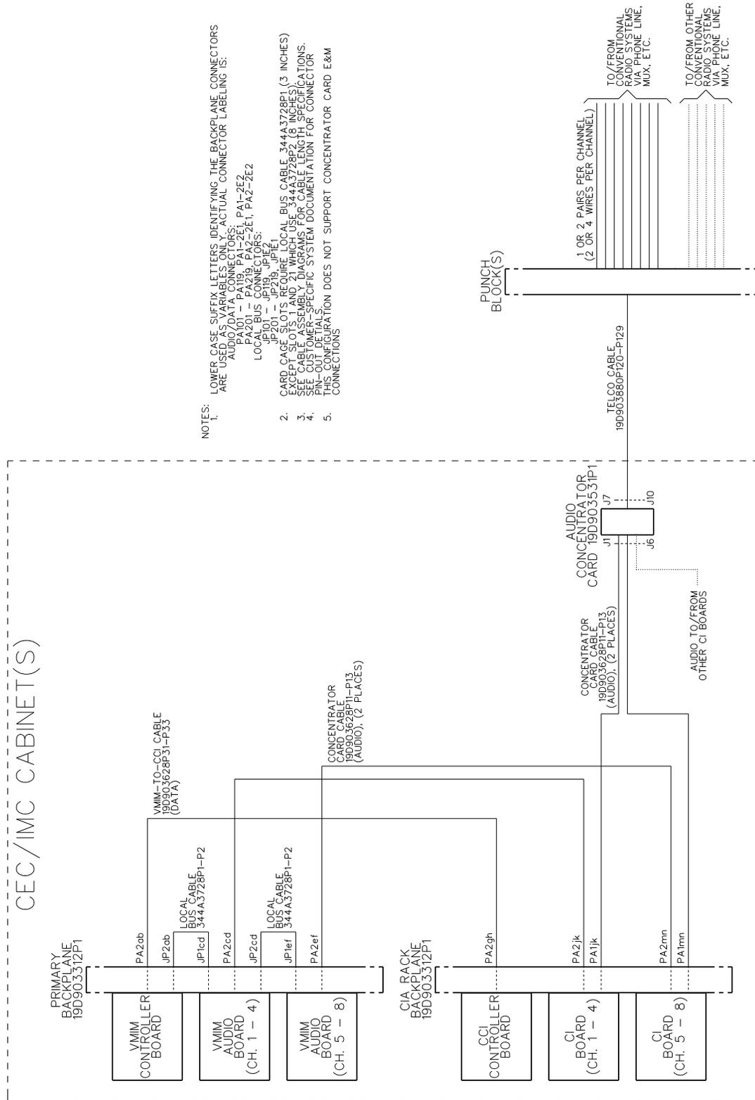
Figure 7 - Typical VMIM/CIA Rack Cable Interconnections Using Audio Concentrator Card 19D903531P1 (8 Channels Shown)
