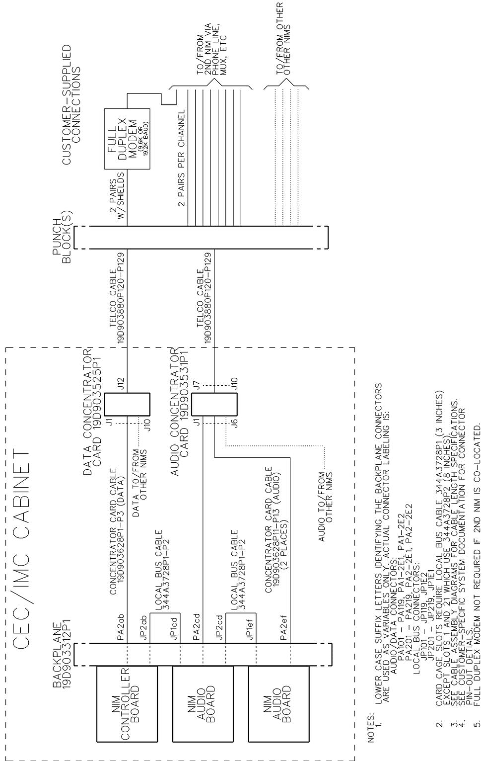
Figure 5 - Typical NIM Cable Interconnections (8 Channels Shown)
