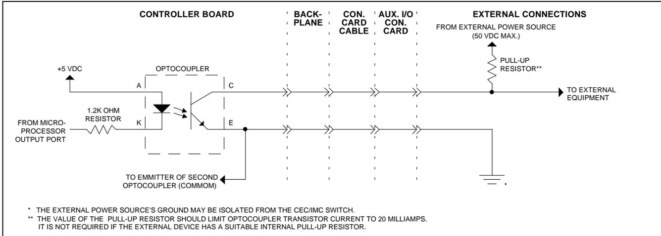
Figure 12 - Auxiliary Output Connection
