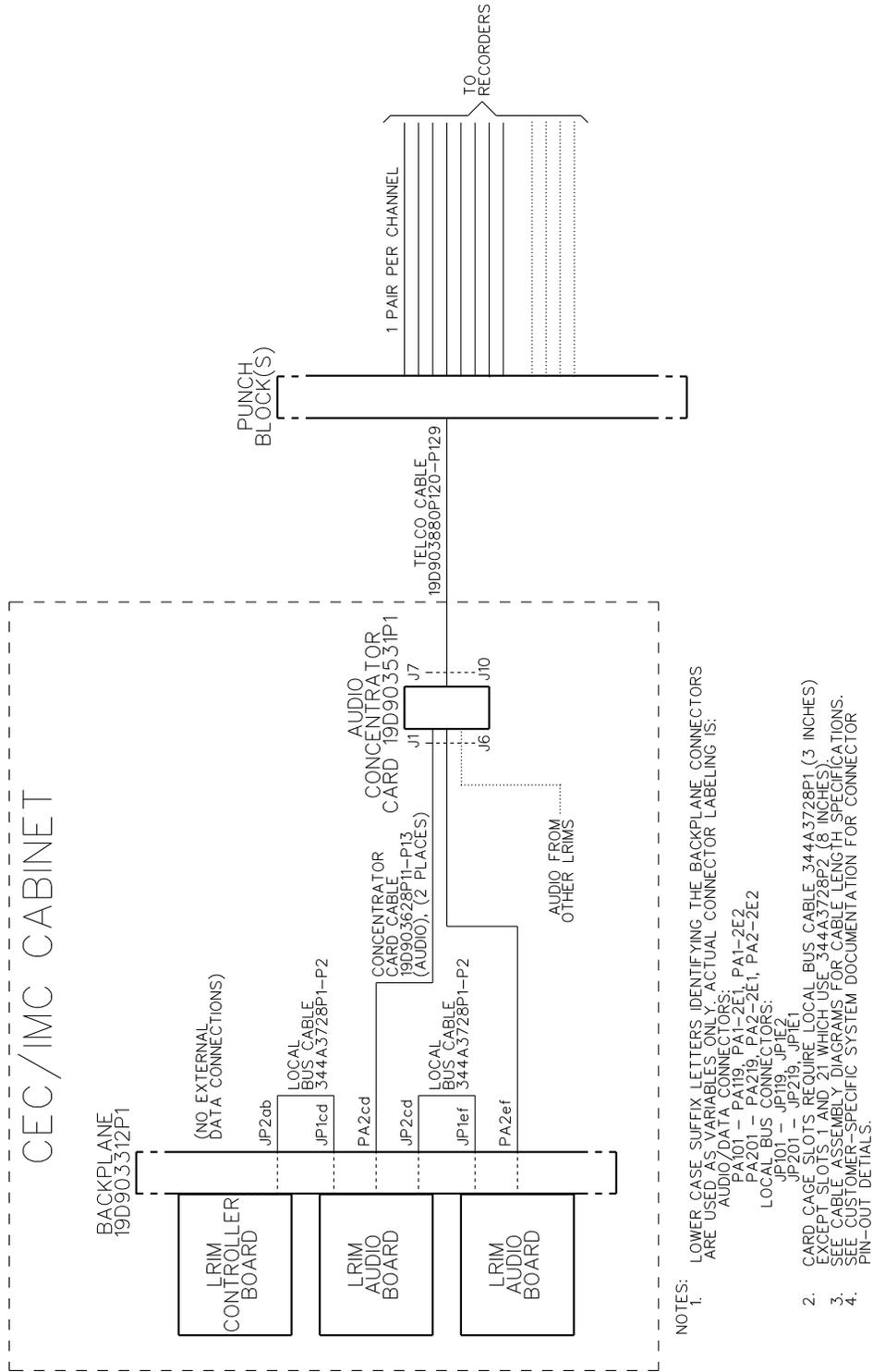
Figure 6 - Typical LRIM Cable Interconnections (8 Channels Shown)
