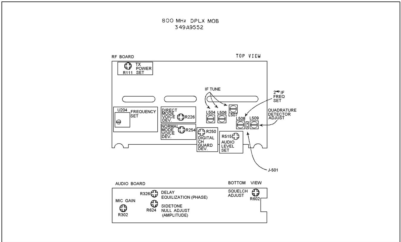
Figure 1- Location of Adjustment Controls
