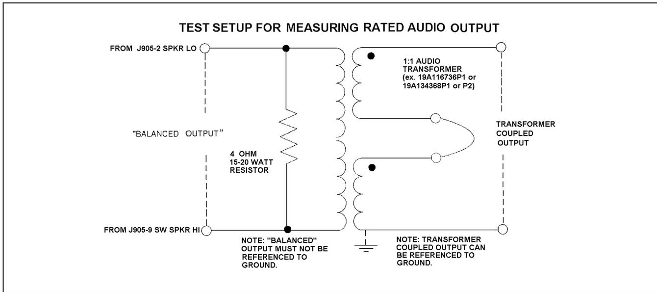
Figure 2 - Audio Output Test Set-up Diagram
