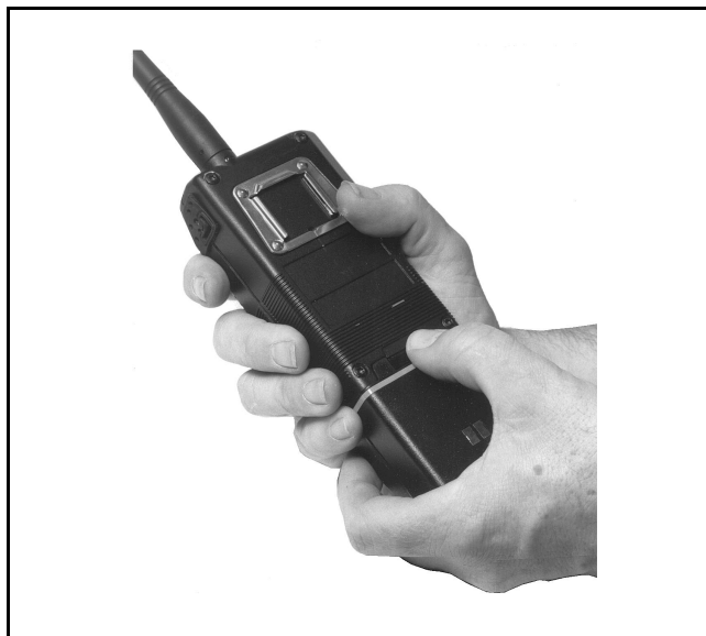
Figure 3 - Removing the Battery Pack
