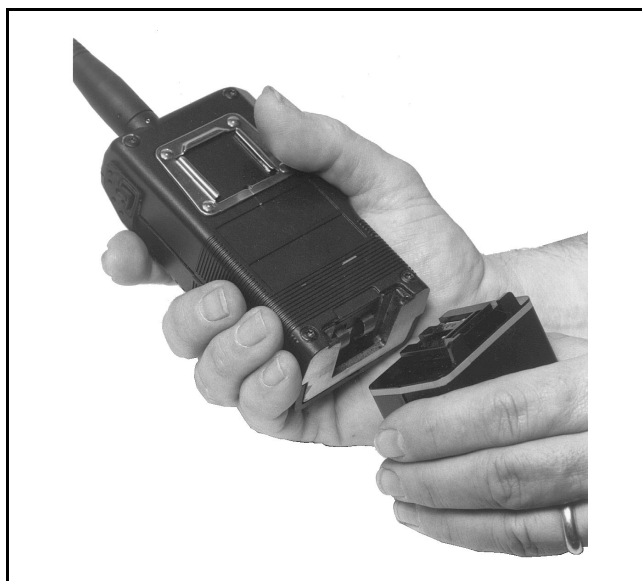
Figure 4 - Installing the Battery Pack
