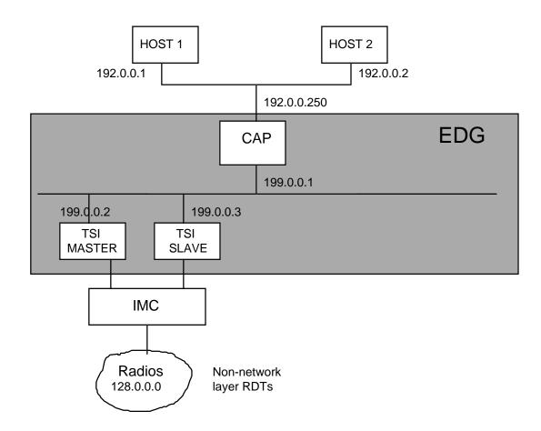
Example 1 represents a TSI Master/Slave configuration with two external IP hosts. Since the IP hosts are on the CAP's local external network (they both have the same class C network ID as the CAP), a CAP external routing table is not required.
