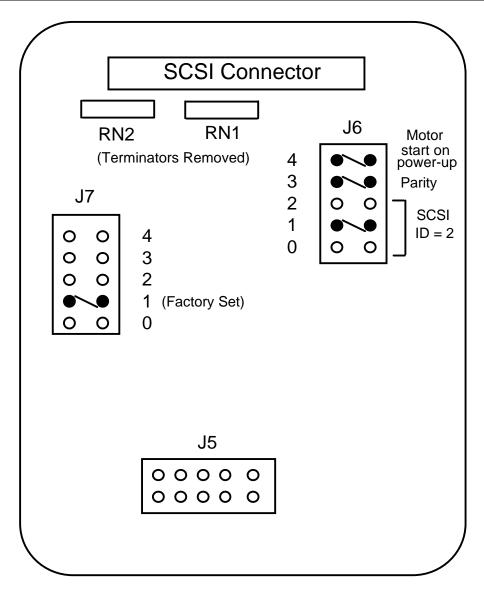
Figure B.6 - Maxtor MXT-1240S Hard Disk
