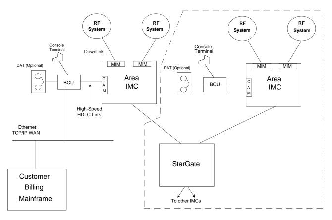
The dotted lines enclose one optional setup for a StarGate (multi-node) billing architecture.
