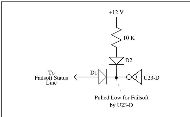
Figure 2 - GETC Failsoft Enable Circuit
