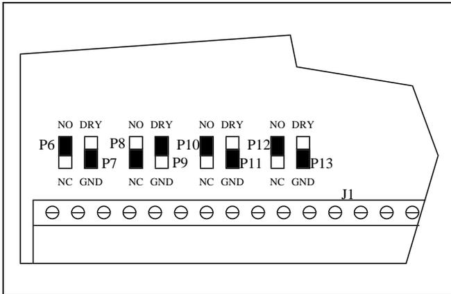
Figure 1 - Jumper Locations and Positions
