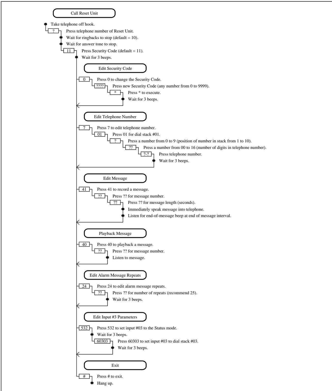
Figure 5 - Programming by Telephone
