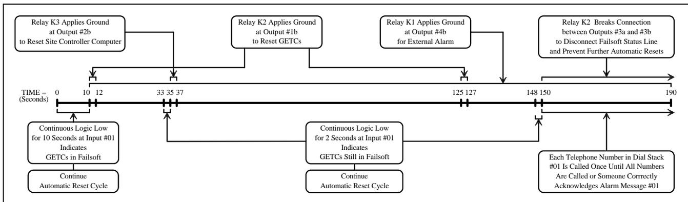
Figure 7 - Automatic Reset Cycle
