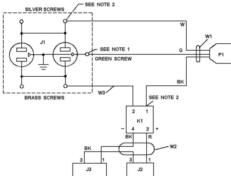
AC Relay Panel Interconnection Diagram
