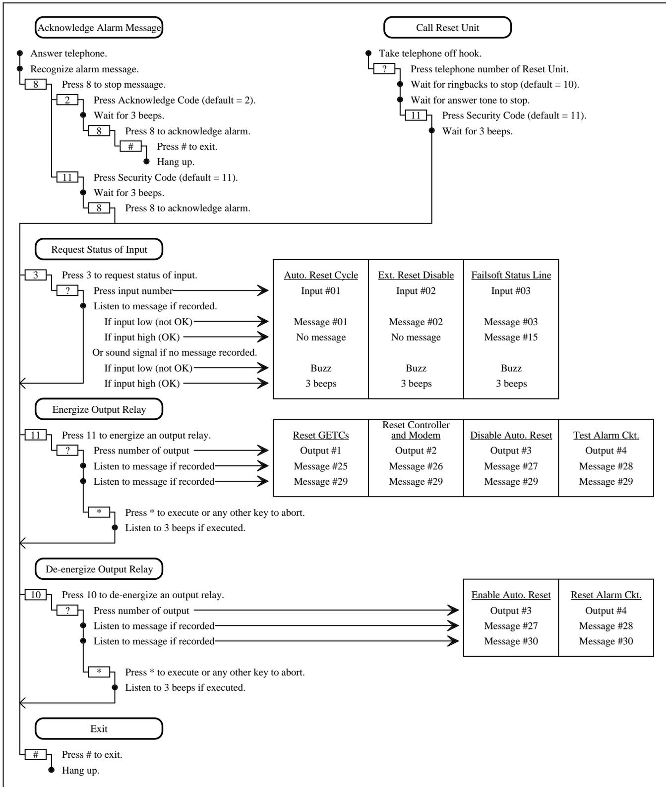
Figure 8 - Operations by Telephone
