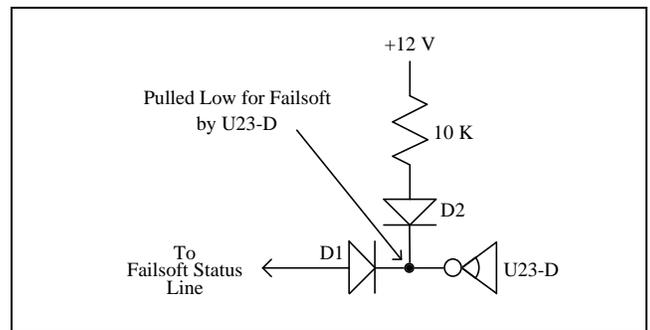
Figure 6 - GETC Failsoft Enable Circuit
