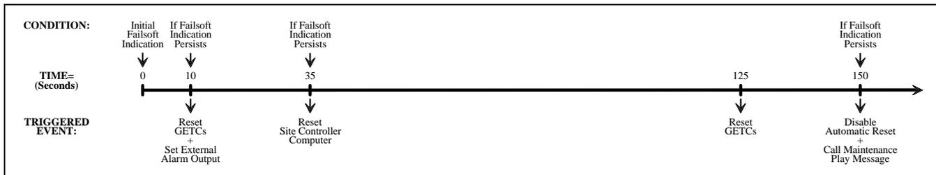
Figure 1 - Simplified Automatic Reset Cycle
