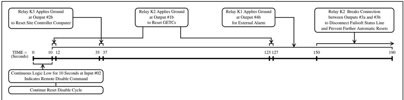
Figure 9 - External Reset Disable Cycle
