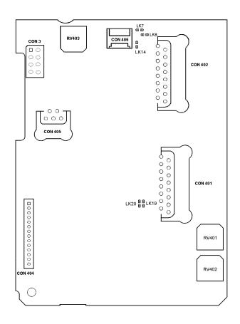
Figure 4 - Radio Printed Wiring Board Layout (4/16 Channel Version)
