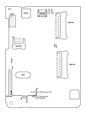
Figure 2 - Radio Printed Wiring Board Layout (10 Channel Version)
