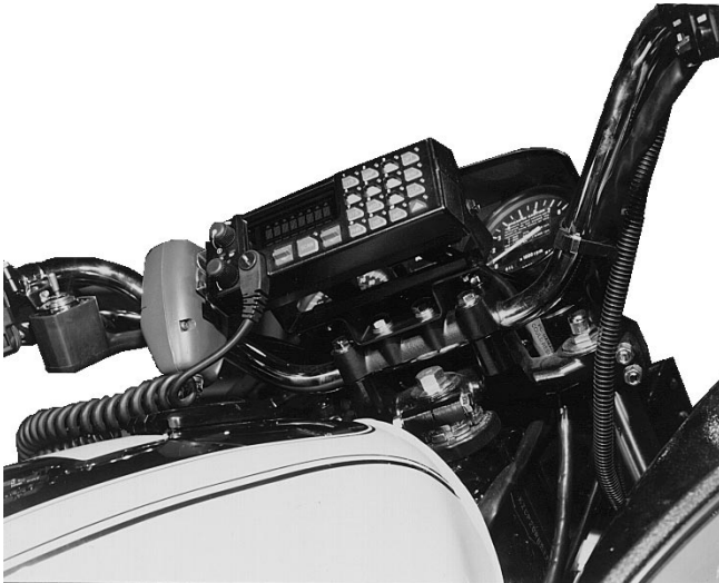
Figure 9 - Typical Control Unit Installation
