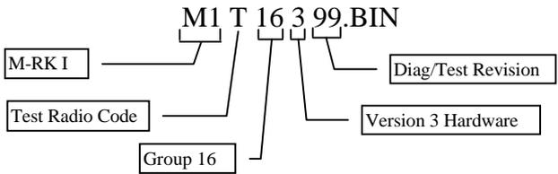
For an ORION radio with Version 3 hardware, use file:
