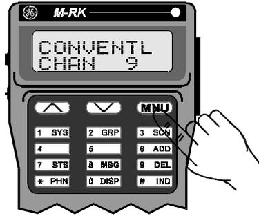
Once accessed, the Diagnostic Radio Menu displays the current diagnostic variable on the top line of the display followed by a value
