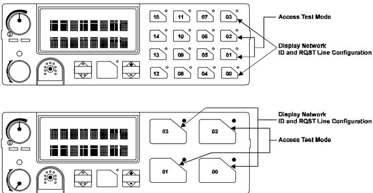
**Figure 6 - Access Control Unit Test Mode**
