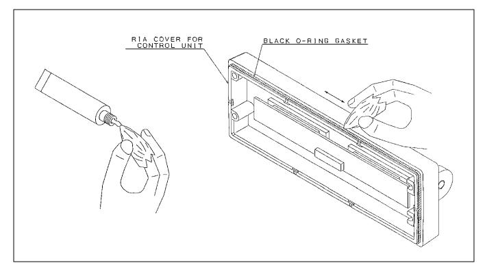
Figure 1B - Remote Mount Control Unit "O-Ring" Lubrication
