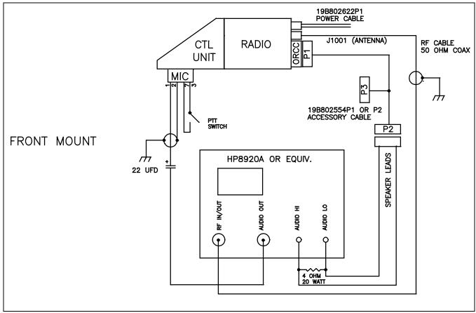
Figure 5 - Typical ORION Test Configuration
