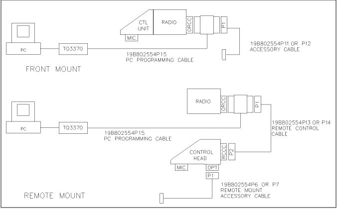
Figure 3 - ORION Programming Configurations (EURO)
