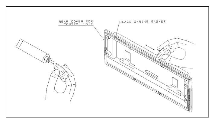
Figure 1A - Front Mount Control Unit "O-Ring" Lubrication
