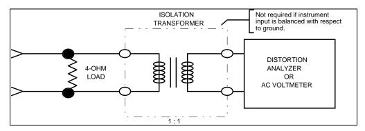
Figure 4 - Audio Isolation Transformer
