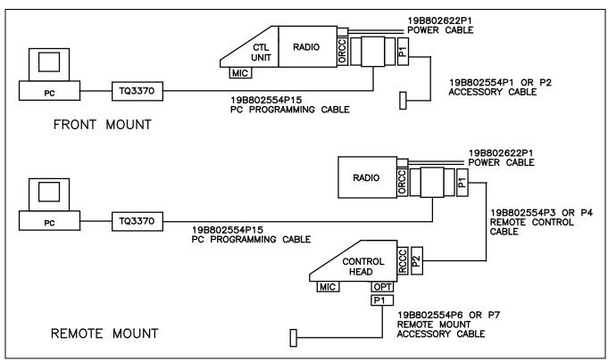
Figure 2 - ORION Programming Configurations (USA)
