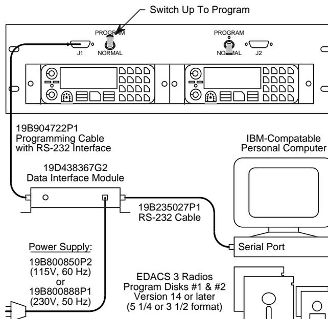
Figure 10 - Programming Setup
