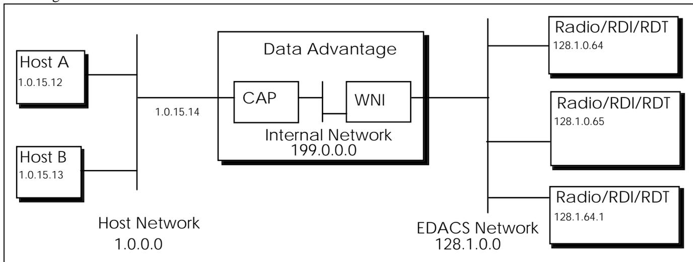
Figure 4 - An IP host internet with individual addresses assigned
