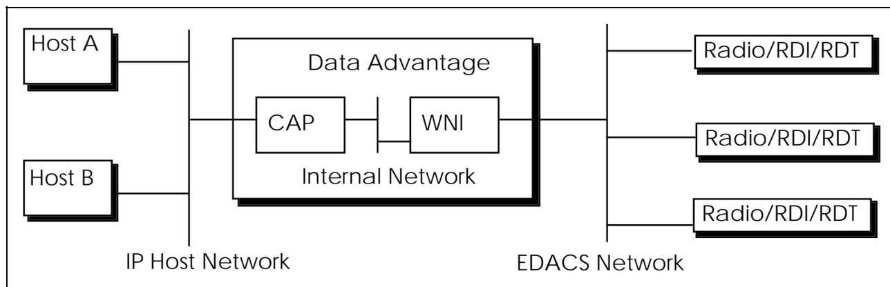
Figure 2 - An IP host internet with no IP Addresses
