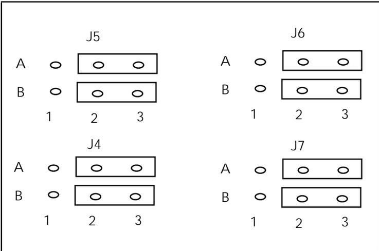
Figure 7 - Jumping SCI-232 for DTE
