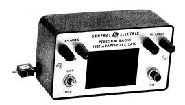
General Electric Test Adaptor Model 4EX12A10 is designed to provide audio connections for servicing MASTR PR Model transmitters and receivers. The transmitter and receiver audio circuits are connected to the audio jacks on the front of the Test Adaptor by mean of a cable that connects to the accessory jack on the radio. The audio jacks are mounted to permit use of a standard dual-banana plug.
