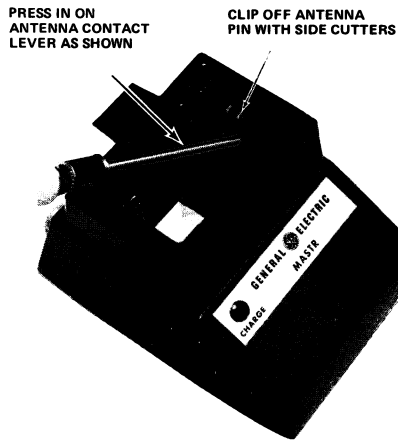
Figure 3 - Disabling the External Antenna Connection
