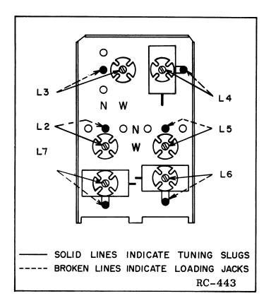
FIG. 2 Location of Tuning Slugs and Jacks, 290-kc IF Transformer - T303
