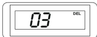
To remove the lock-out condition from a channel, manually select the channel and press **(L/O)** again.
