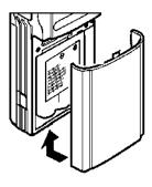
Push the side latches forward to lock the cover into place.
