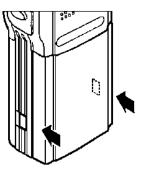
Remove the cover by sliding it down and away from the radio.
