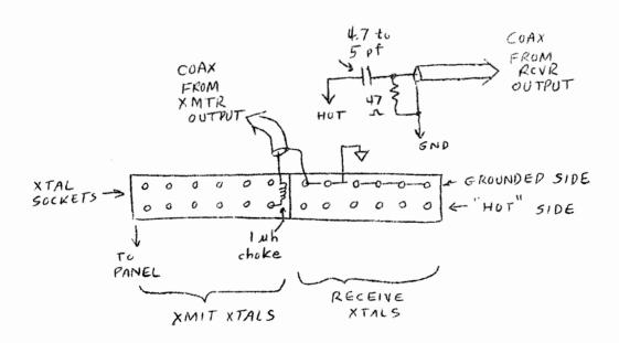
Note that the rear pin of each receive crystal socket is grounded; thus providing a convenient ground for both coaxes if channel 6 is used for Channelized operation.
