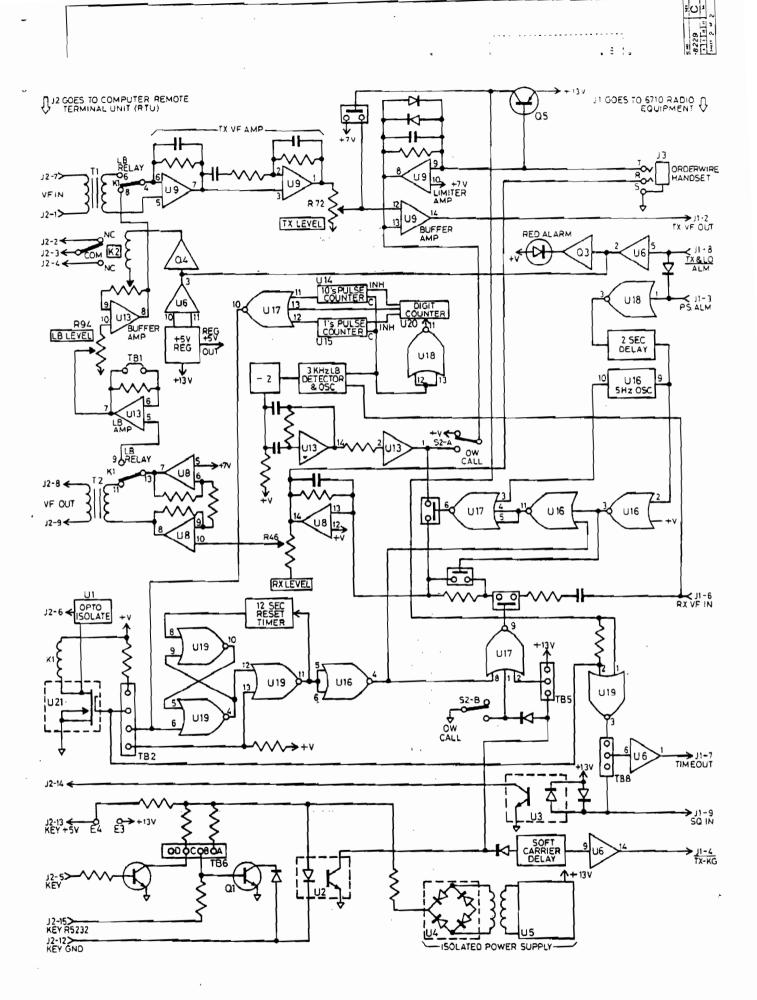
Figure 1 Interface 002-0246-XX Module Block Diagram
