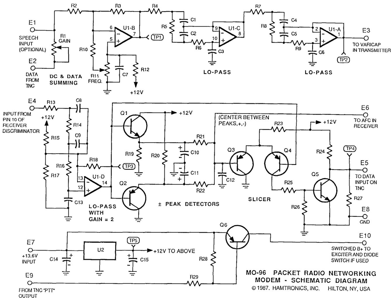
**MO-96 PACKET RADIO NETWORKING MODEM - SCHEMATIC DIAGRAM**
